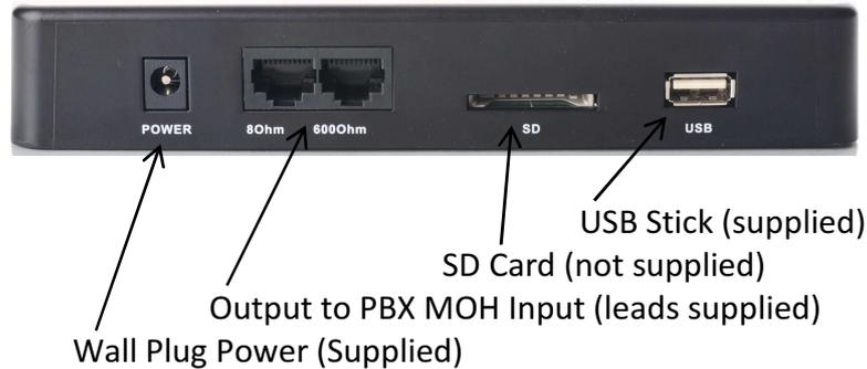
1. Connect power & check MOH Player is working (press and hold Speaker Key to hear standard greeting pre-installed).
