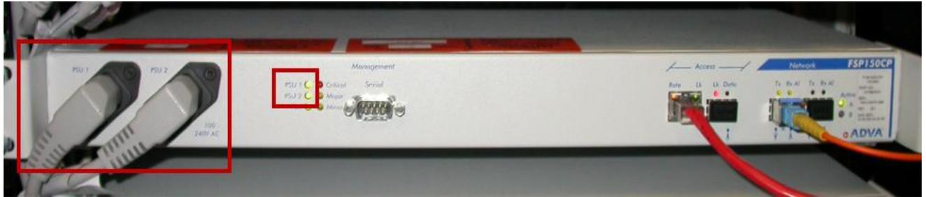
Check that both power cables are plugged in correctly, and that the alarm lights for the PSUs are solid green.
